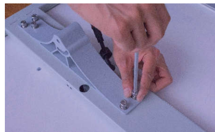
3.Fix the Vertical Bracket on the Solar Panel.
