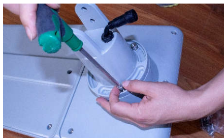
2.Put the Horizontal Bracket on the light body and fasten the screws.
