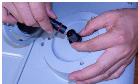
1.Connect the quadripuntal connectors of Horizontal Bracket&light body together
